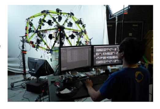
A photogrammetry rigging prototype to take high resolution, 3D images of items
